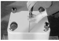
Remove the 4 retaining screws from the bottom cover.
