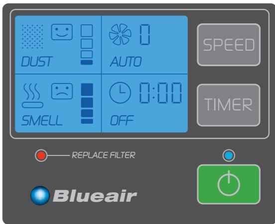
**POWER ON/OFF.** Press the green POWER key to turn the unit on and off. The unit automatically runs on the highest speed for five minutes after it is turned on to provide fast initial cleaning and then switches to Auto Mode.
