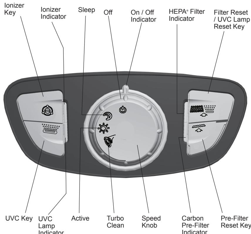
Fig. 3 - Air Purifier Control Area
